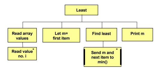
Entry of values is made in a loop. Then we set the variable m equal to the first item of the array. In the loop 'Find least' we send m and the next item to the function min(). The return value is stored in the variable m. Since we use m to store the returned value, m will all the time contain the least of the items compared so far. At completion of the loop we print the m value, which now is the least of all array items.
